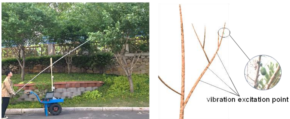
Fig. 7 - Schematic diagram of the harvesting trials
