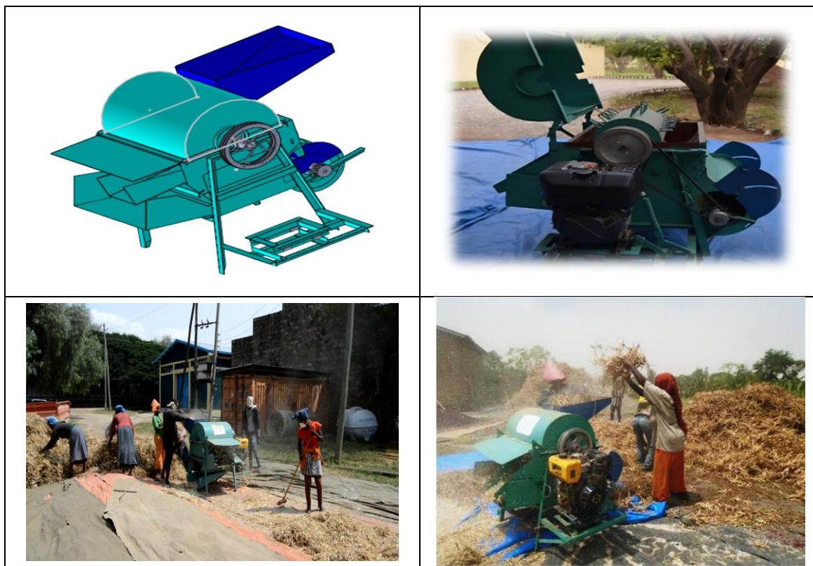
Fig. 1 – MARC Bean thresher schematic diagram and participatory evaluation assessment
