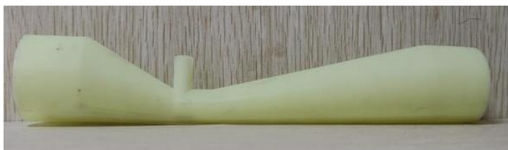
Fig. 10 - Physical drawing of S5L1 venturi aerator
