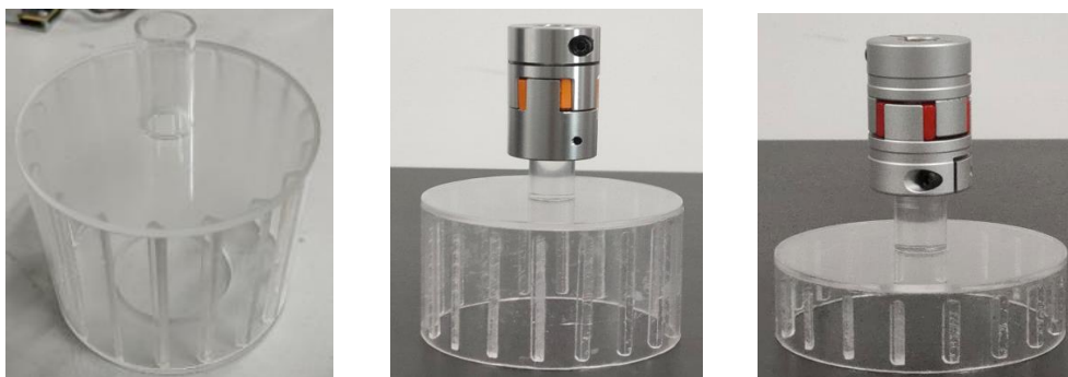
Fig. 15 - Three different lengths of the drum-type sprouted brown rice machine tank (left: 75 mm mid: 50 mm right: 25 mm)
