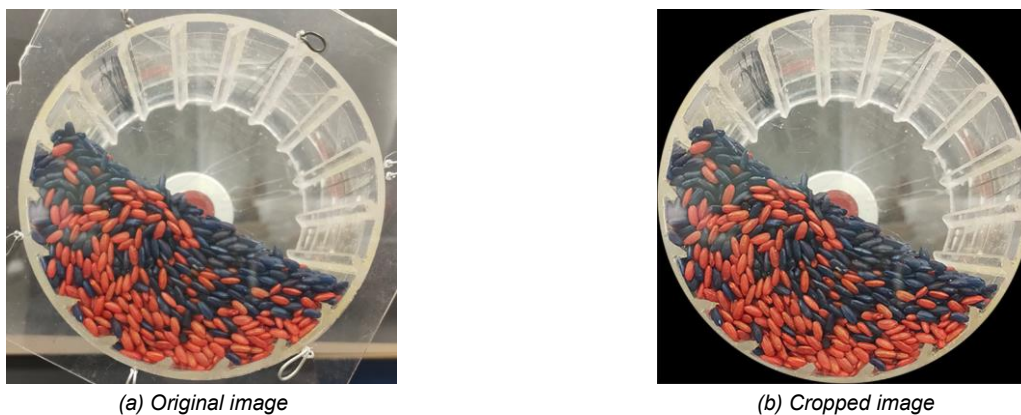
Fig. 20 - Image of particle blending at a mixing time of 5 s
