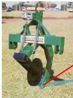
(a) Digging and loosening cassava harvester
