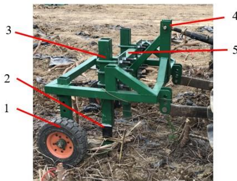
Fig. 3 - Loosening shovel resistance test system
