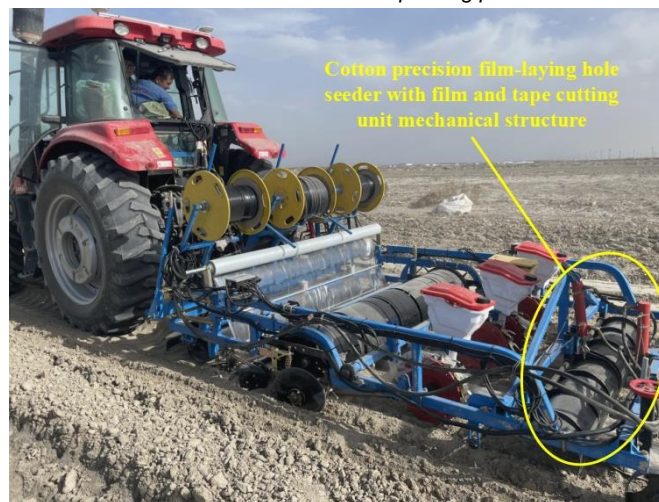
(b) Installation position of unit mechanical structure
