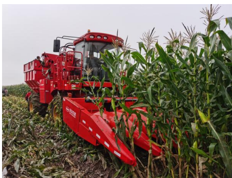
Fig. 5 - Field operation of 4YX-6 fresh corn combine harvester
