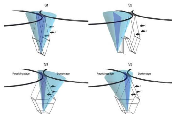
Fig. 6 - Side scan sonar for biomass estimation of tuna during transfers, (Puig-Pons *et al.*, 2019)
