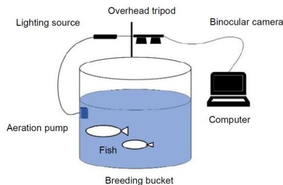
**Fig. 2 - Experimental stand scheme** (Zhou *et al.*, 2023)
