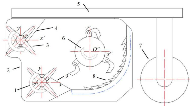
**Fig. 3 - Simplified diagram of the branch crusher of the double-roller picking and feeding mechanism**
