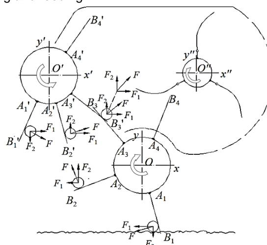
Fig. 2 - Kinetic analysis of the double-roller picking device
