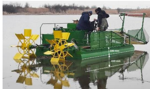
Fig. 4 - Measuring the draft of the boat in different conditions
