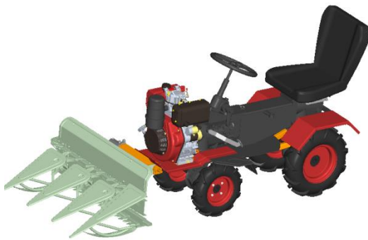
Fig. 1 – Overall highland barley harvesting and binding machine
