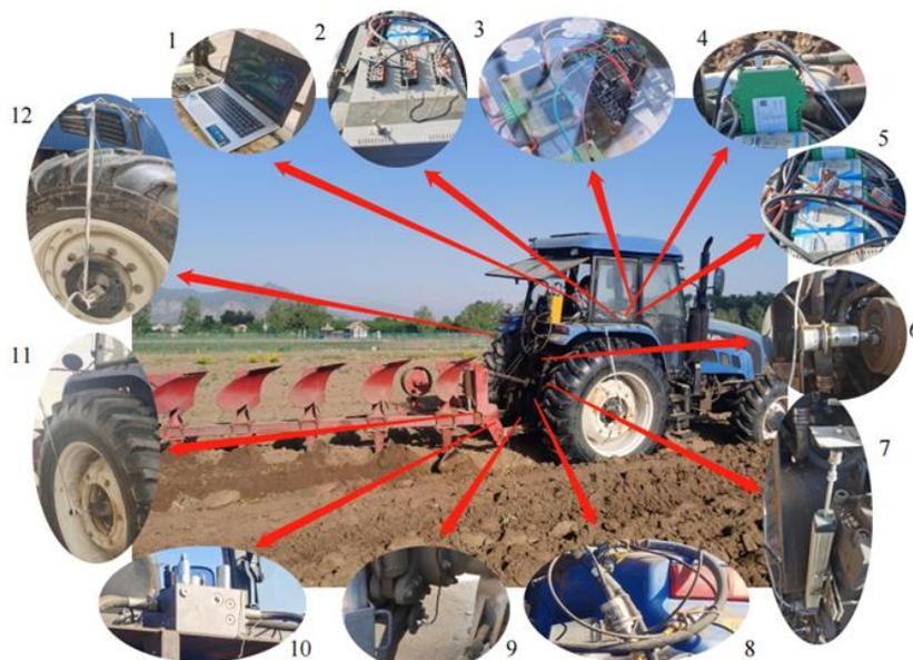
**Fig. 5 – Field test platform of tractor electro-hydraulic hitch control system**
