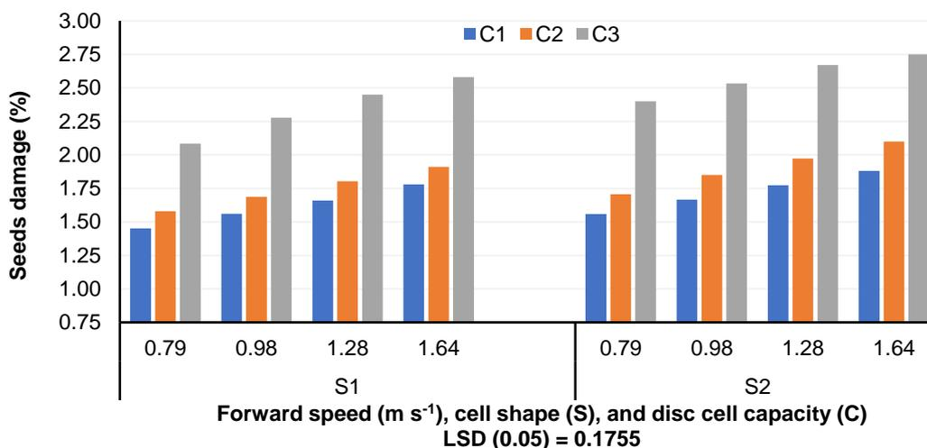
Fig. 7 – Effect of forward speed, cell shapes, and disc cell capacity on seeds damage percentage
