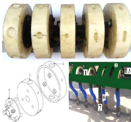
**Fig. 2 – The seed metering device**
