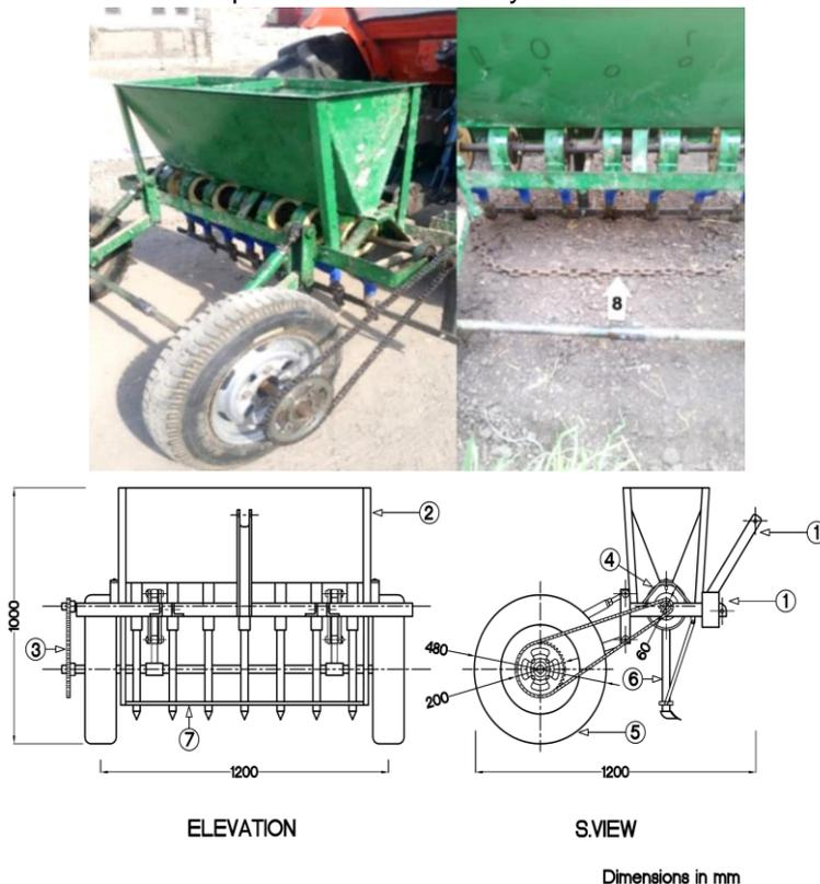
**Fig. 1 – Photo, elevation and side views of the seed drill**
