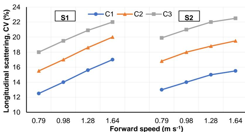
Fig. 9 – Effect of forward speed, cell shape, and disc cell capacity on longitudinal scattering
