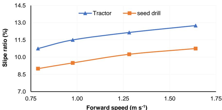
Fig. 6 – Effect of forward speed on slip ratio
