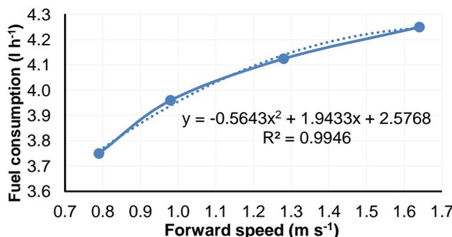
Fig. 4 – Effect of forward speed on fuel consumption
