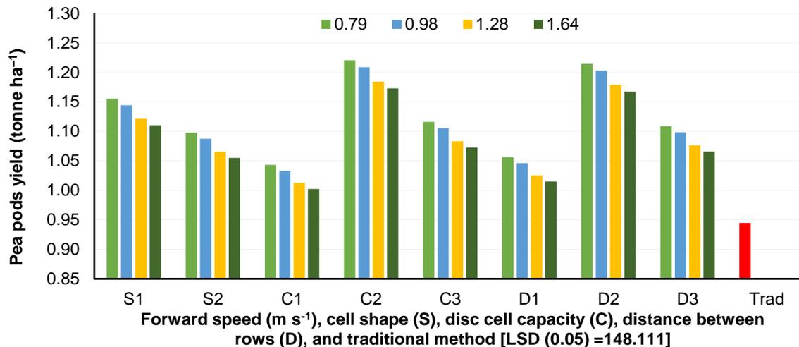
Fig. 10 – Effect of forward speed, cell shape, disc cell capacity, and distance between rows on the pea pods yield
