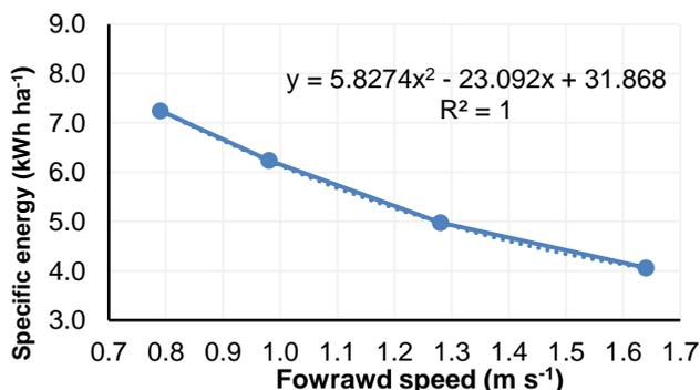
Fig. 5 – Effect of forward speed on specific energy
