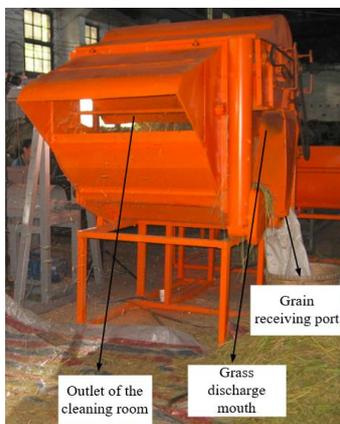
Fig. 6 - Material collecting area after experiment
