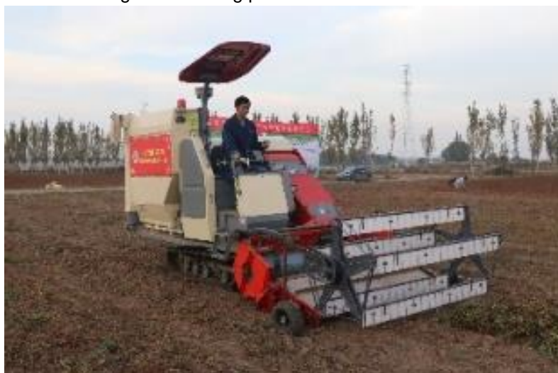
Fig. 7 - 4LJQ-1.5 two-stage buckwheat picker combine harvester
