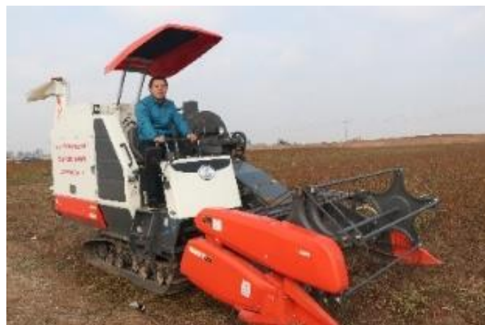
Fig. 6 - 4LZQ-1.5 crawler buckwheat combine harvester
