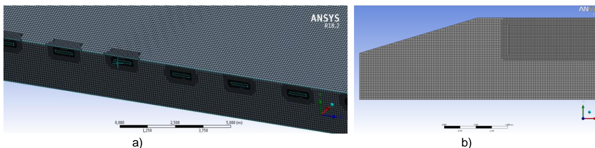
Fig. 3 – Net of poultry house on the side (a) and on the rear end (b)
