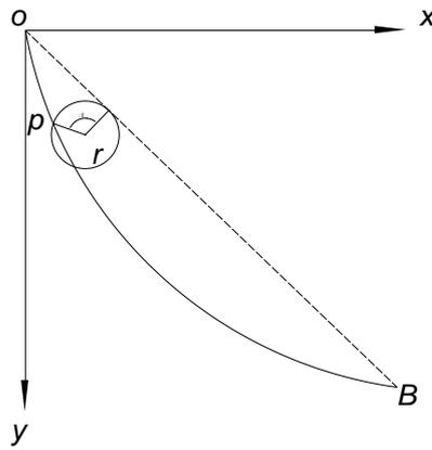
Fig. 2 - Geometric meaning of brachistochrone
