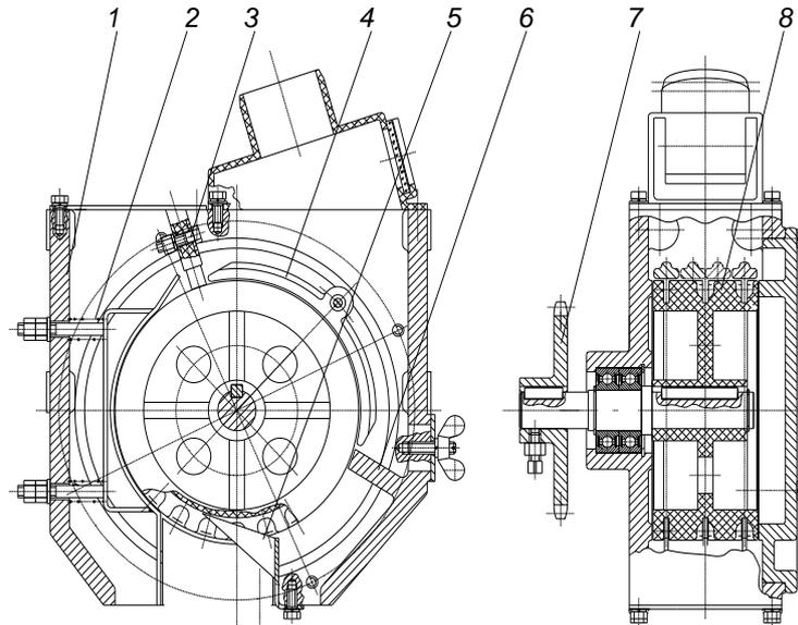
**Fig. 1 - Structure of precision seed metering device**
