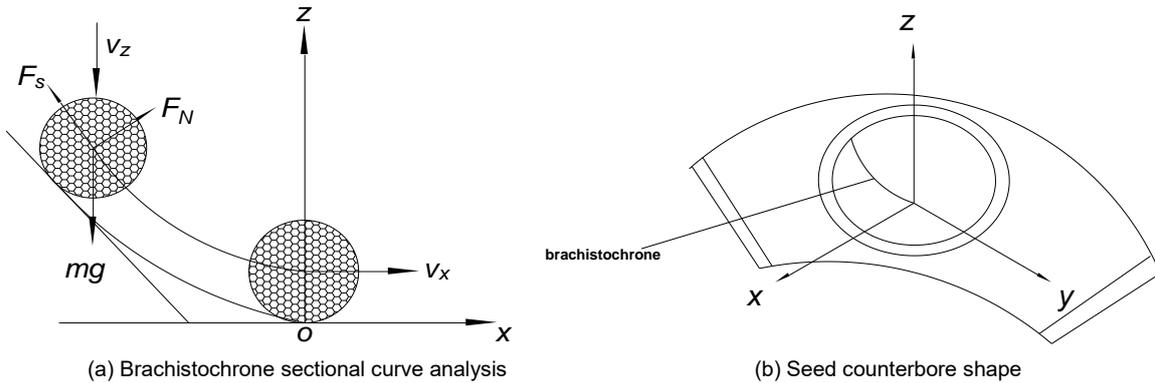
Fig. 3 - Analysis of brachistochrone sectional curve
