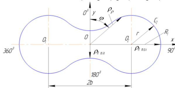
Fig. 2 – Scheme to explain the  $\rho_R$  polar radius as a parameter of rotor geometry
