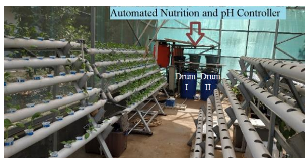
Fig. 1 - Automated Nutrition and pH Controller Equipment for Hydroponic Plant Cultivation
