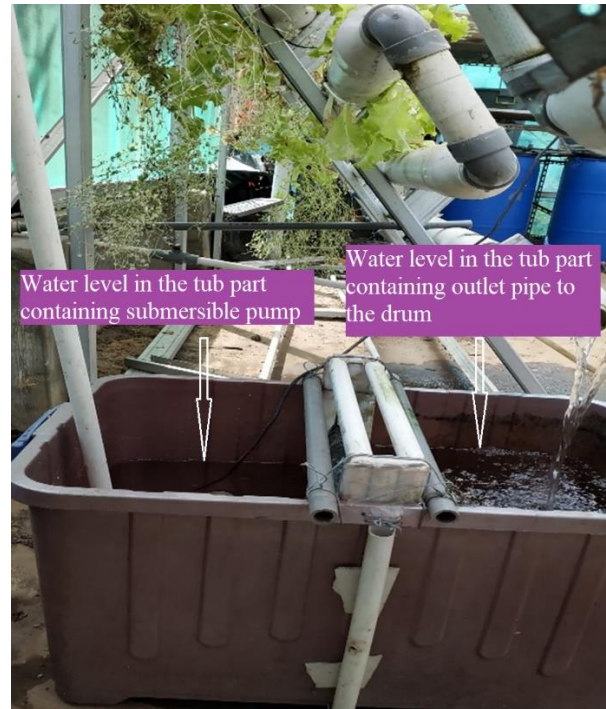
Fig. 4 - Nutrient solution level in the tub-part containing submersible pump (left) and outlet pipe to the drum (right)
