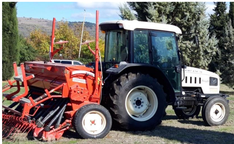
Fig. 2 – Machine-tractor unit with mounted row seeder
