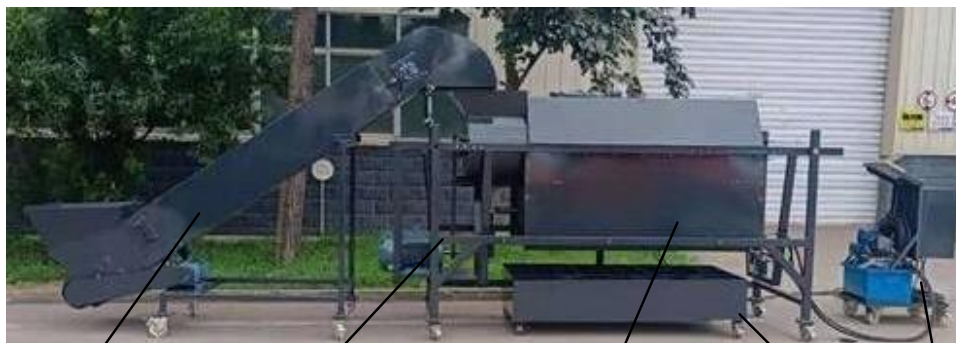
The feeding device Frame of threshing test stand Threshing and separating device Picking device Control device
