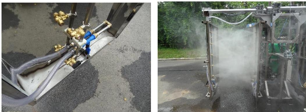
Fig. 14 – Testing the spraying machine with solution recovery system equipped with Venturi injectors
