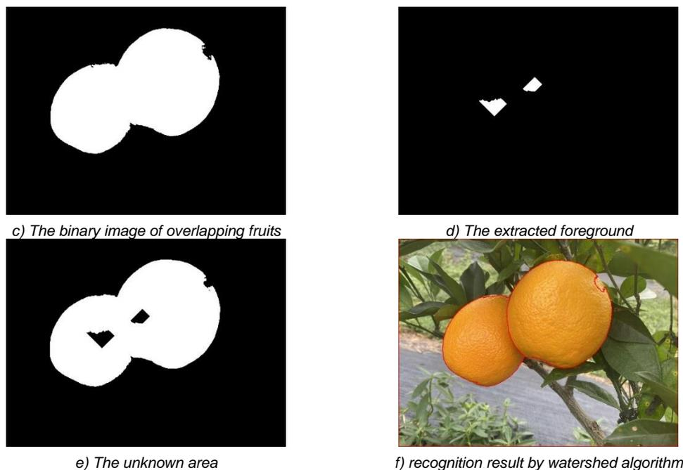
**Fig. 3 – Separating overlapping fruits based on watershed algorithm**
