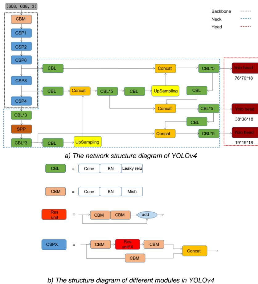
Fig. 4 - The architecture of YOLOv4 network
