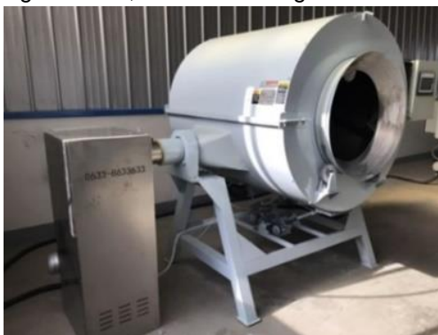
Fig. 14 - Experimental prototype of hot air tea roasting machine
