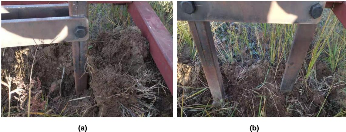
**Fig. 10 - Coupling procedure between the grassland surface and ditching parts:**
