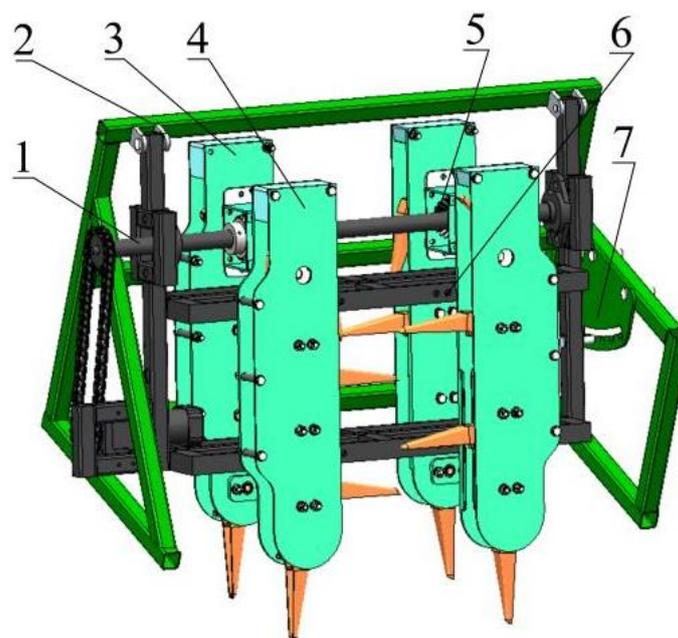
**Fig. 1 - Structure diagram of double-chain finger grain lifter**
