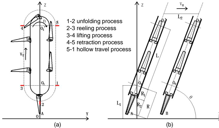
**Fig. 3 - Kinematic model of working process**
