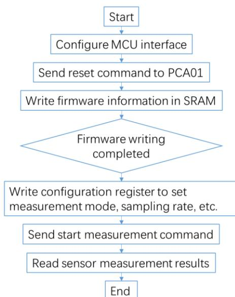
Fig. 5 - Flow chart of MCU software program
