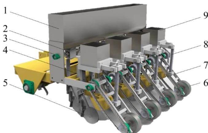
**Fig. 1 - Mechanical structure diagram of the fertilizer applicator**
