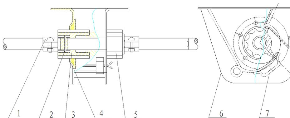
**Fig. 3 - External grooved wheel fertilizer spreader**
