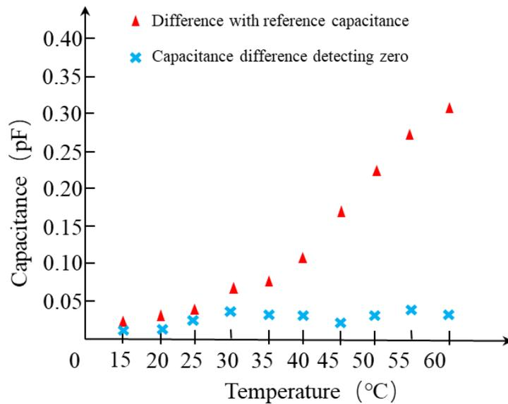
Fig. 6 - Influence of temperature on capacitance output
