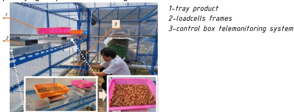
Fig. 3 – Telemonitoring devices integrated into the solar dryer
