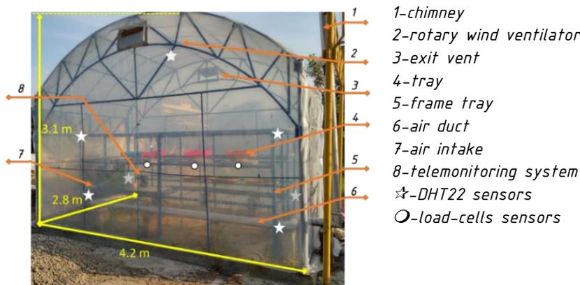
Fig. 1 – Solar dryer developed in this study
