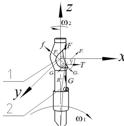
**Fig. 5 - Stress analysis of bud seeds in the process of seed-delivery**
