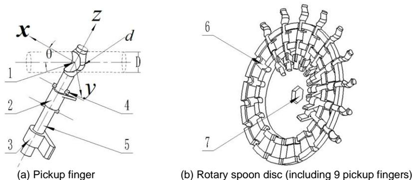
**Fig. 2 - Diagram of pickup finger**
