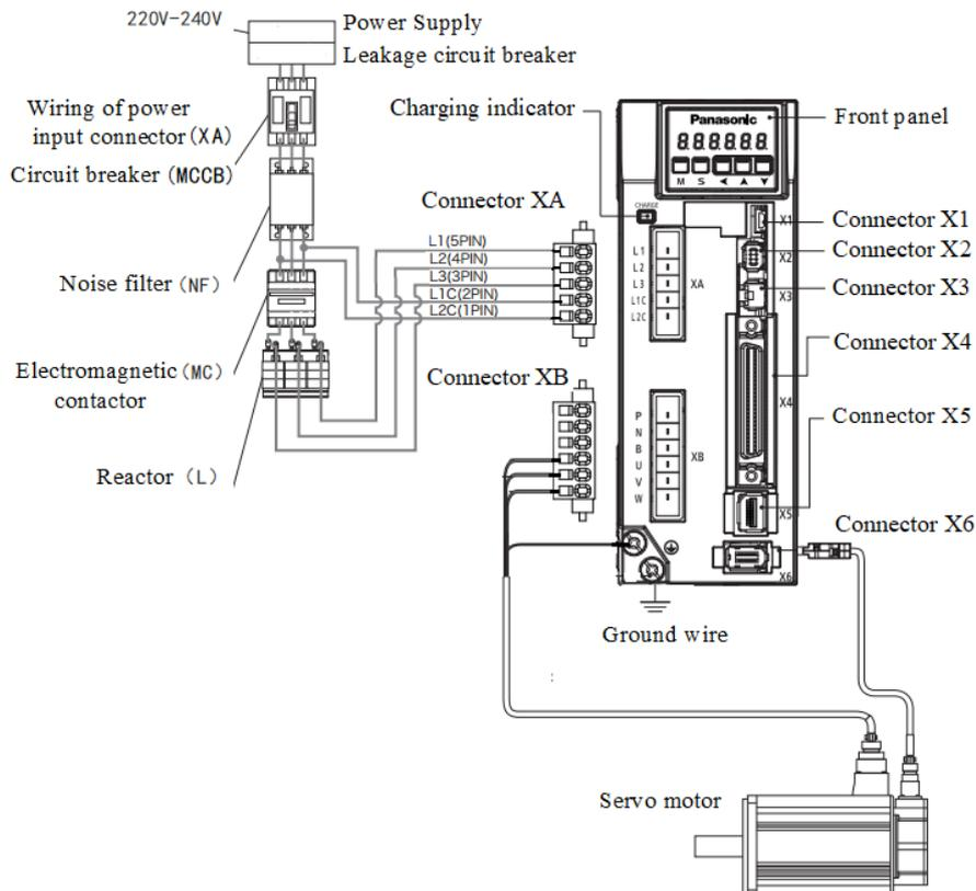
Fig. 4 - Motor driver and peripheral equipment connection diagram
