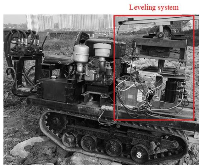
Fig. 7 - The adaptive leveling system testing prototype
