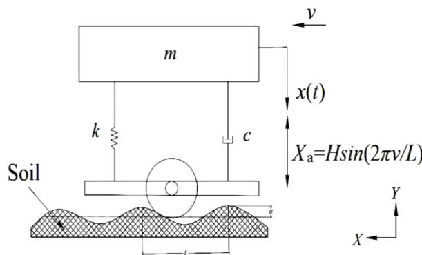
Fig. 2 - Hanging cup transplanter-soil system vibration model
