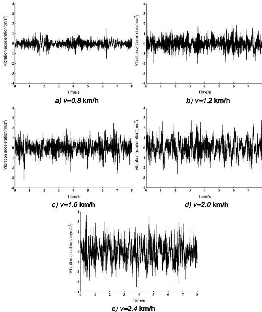
Fig. 5 - Vibration time domain diagram at different speeds
