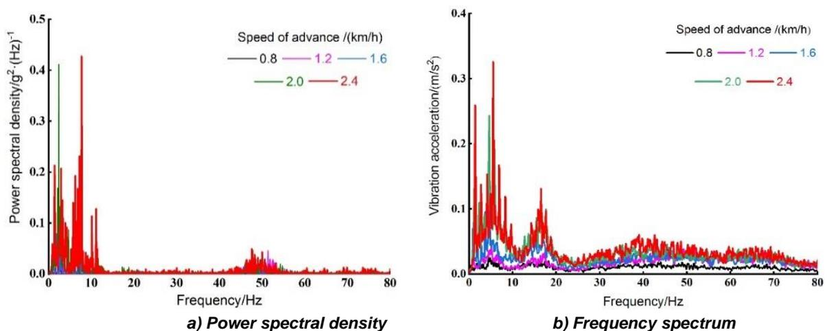
Fig. 6 - Vibration frequency analysis of cup transplanter
