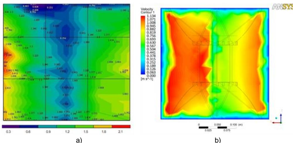
Fig. 8 – Distribution of wind flow velocity (m/s) in front of the WFC
