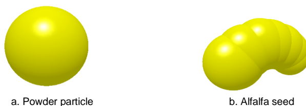
Fig. 1 - Simulation model of alfalfa seeds and powder
