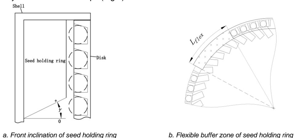
Fig. 4 - Experimental factors of seed holding ring
