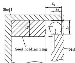
**Fig. 2 - Schematic diagram of seed holding ring**
