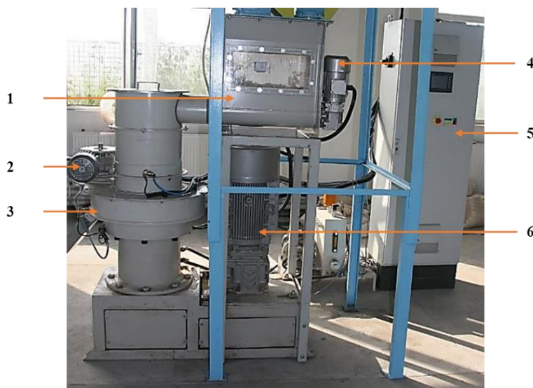
Fig. 1 - Ring die pelleting equipment used for experiments
