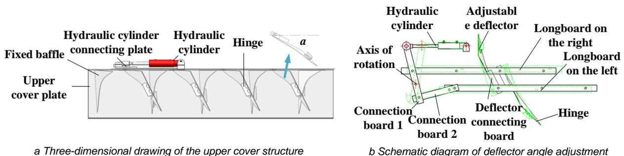
Fig. 5 - Upper cover structure drawing
