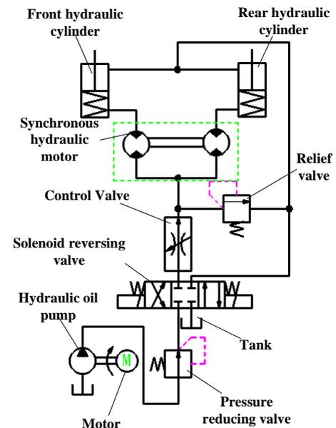
Fig. 4 - Cylinder-concave clearance regulation oil circuit
