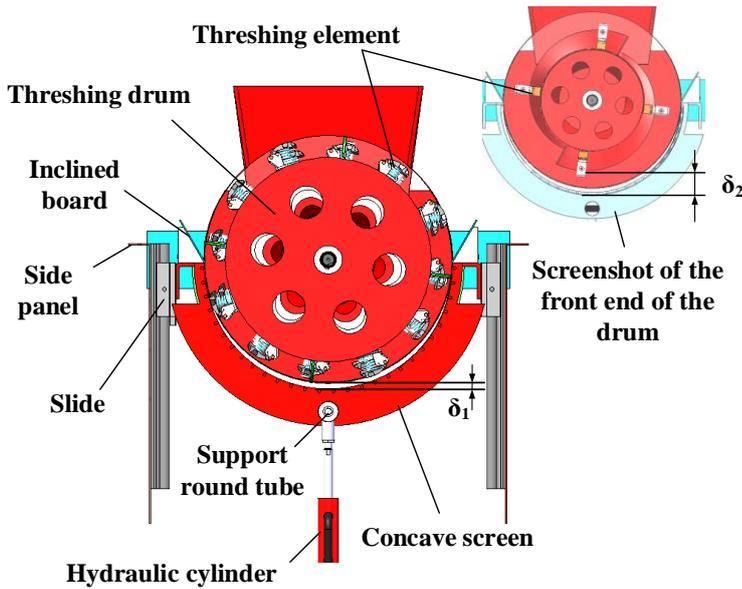
Fig. 3 - Cylinder-concave clearance adjustment design
