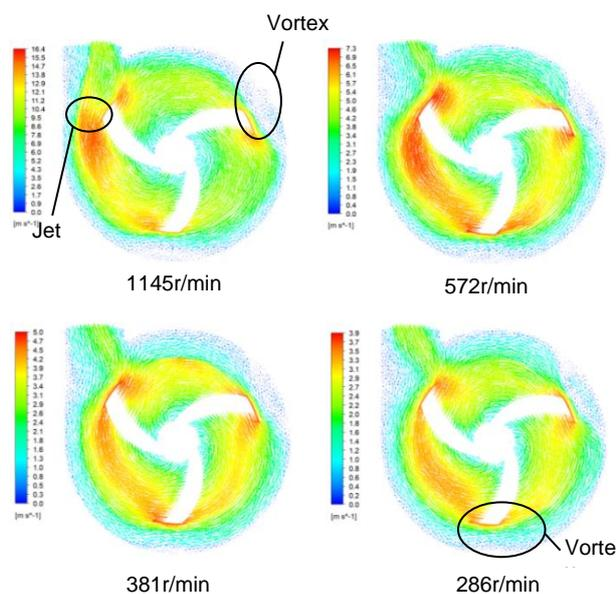
**Fig. 11 - Vector diagram of relative velocity of organic fertilizer particles at different rotational speeds**
