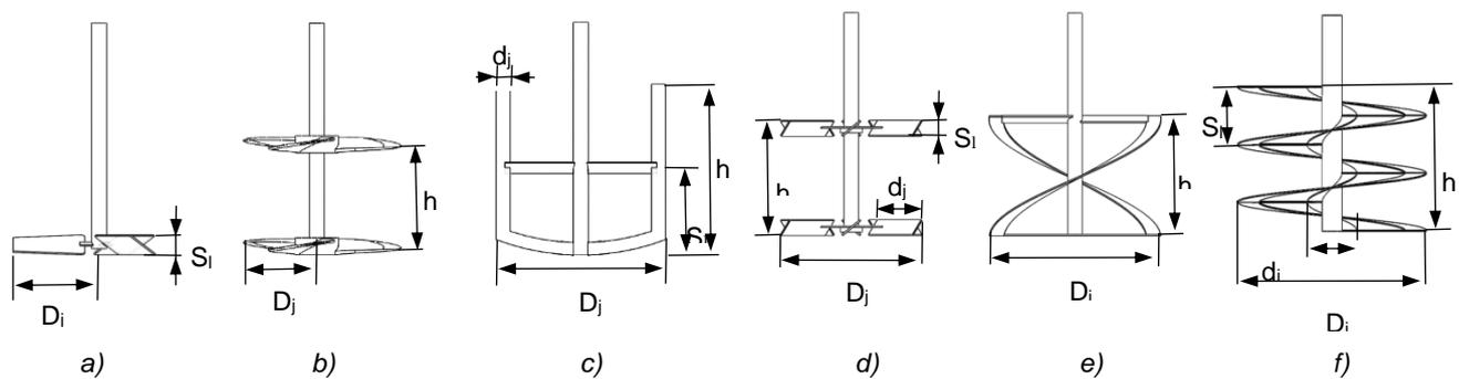
a) Oblique blade type; b) Propelling type; c) Box; d) Folded blade turbine; e) Screw belt; f) Screw-screw
