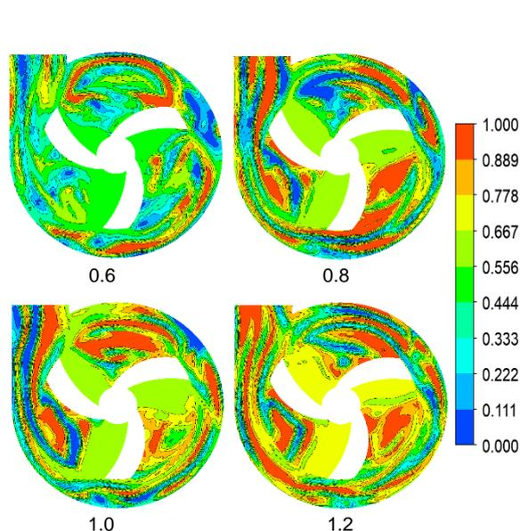
**Fig. 10 - Particle distribution of organic fertilizer with different proportion of fertilizer and water**
