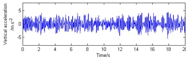
**Fig. 11 - Vertical vibration acceleration of the rear axle**
