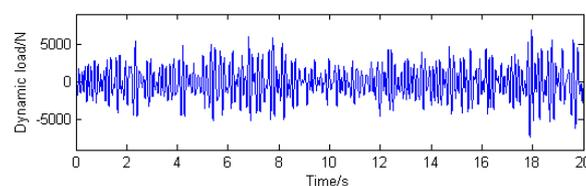
**Fig. 13 - Dynamic load of the tractor rear wheel**
