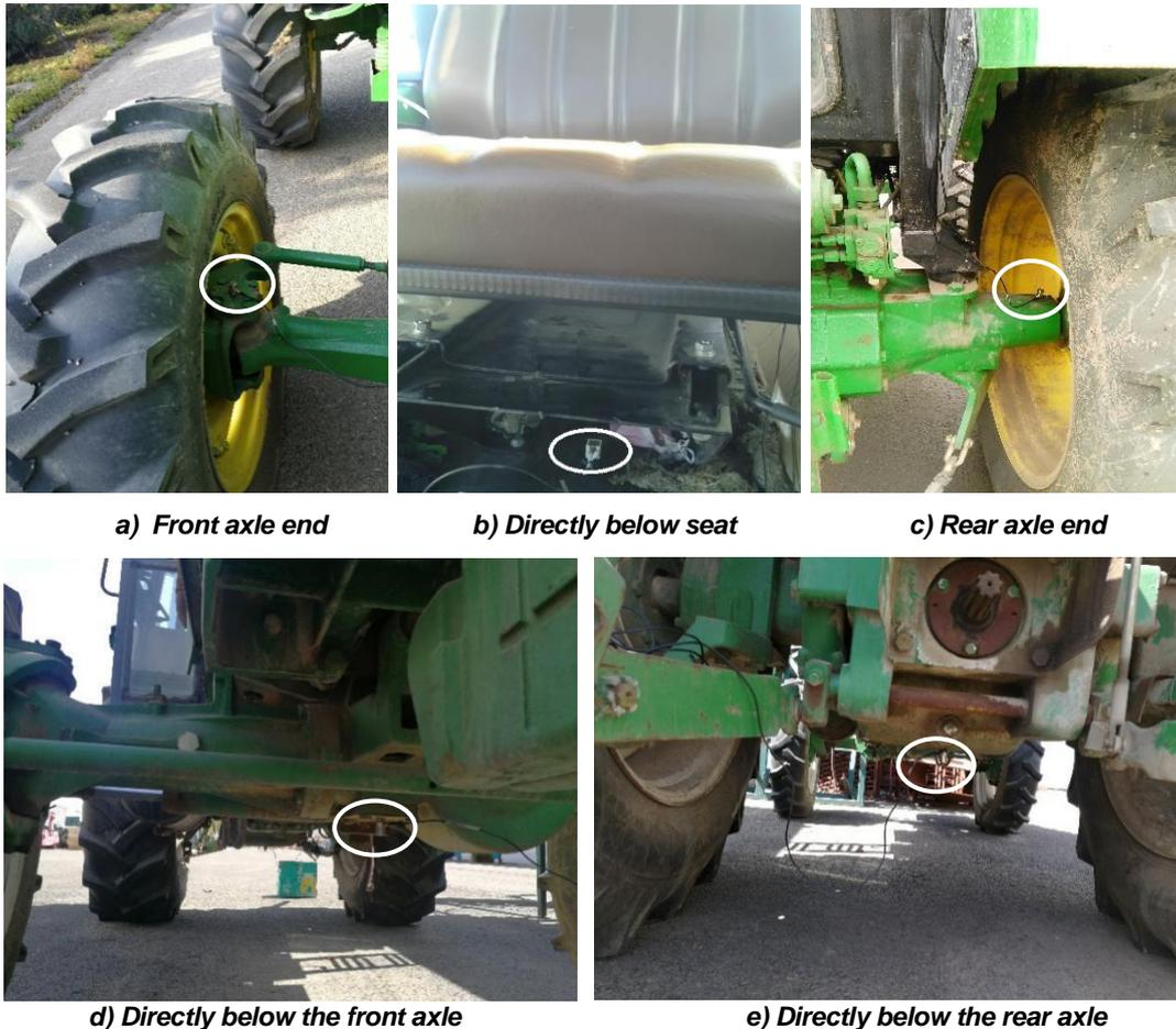
Fig. 3 - Sensor installation positions
