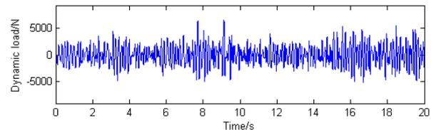
**Fig. 12 - Dynamic load of the tractor front wheel**
