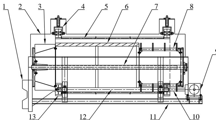
**Fig. 1 - Structure of buckwheat threshing device**
