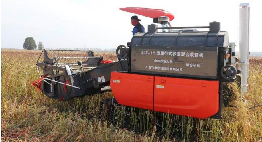
**Fig. 8 - Tracked buckwheat combine harvester prototype**
