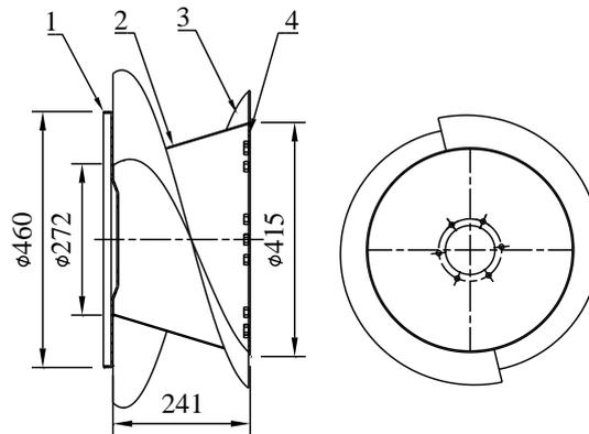
**Fig. 5- Structure of screw feeding device**
