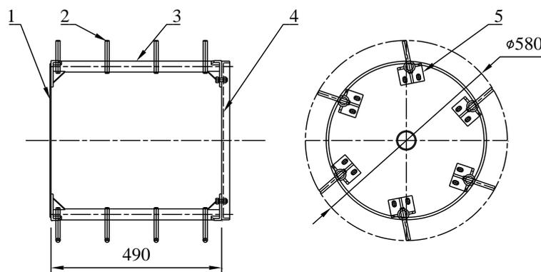
**Fig. 3 - Structure of nail tooth roller**
