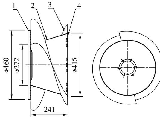
**Fig. 5- Structure of screw feeding device**
