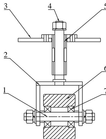
**Fig. 7- Structure of outer roller pressing device**
