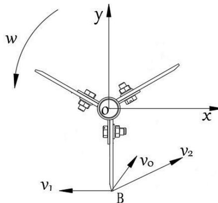
**Fig. 4 - Motion trajectory analysis diagram of the film sweeping device**
