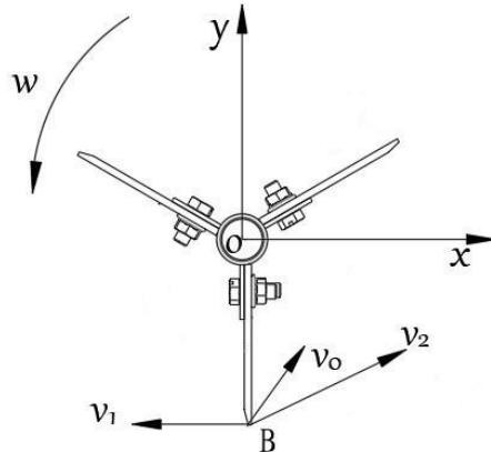
**Fig. 4 - Motion trajectory analysis diagram of the film sweeping device**
