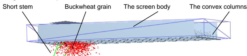
Fig. 5 - Screening simulation process of convex-column sieve
