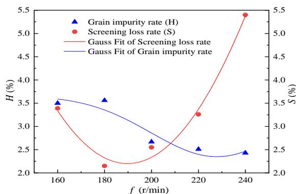
Fig. 11 - Loss rate and impurity rate under different frequency
