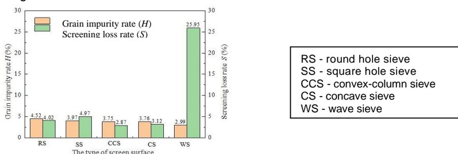
Fig. 7 - Simulation results of five screening surface types
