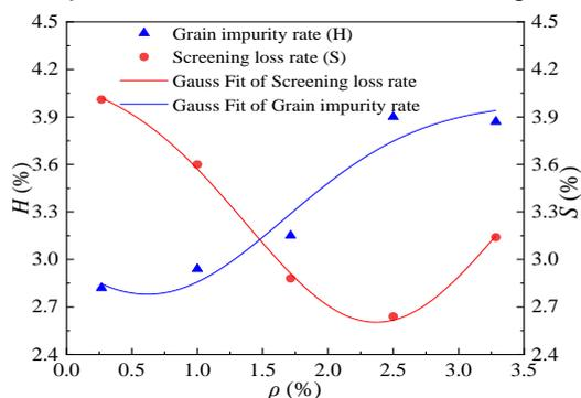
**Fig. 8 - Loss and impurity rates under different convex-column ratio**
