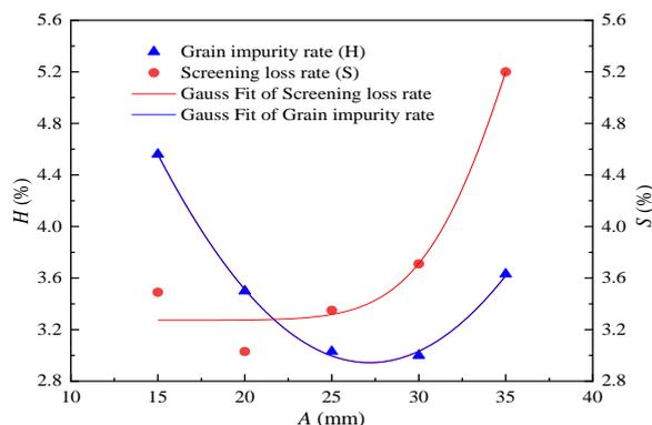
Fig. 10 - Loss rate and impurity content under different amplitude
