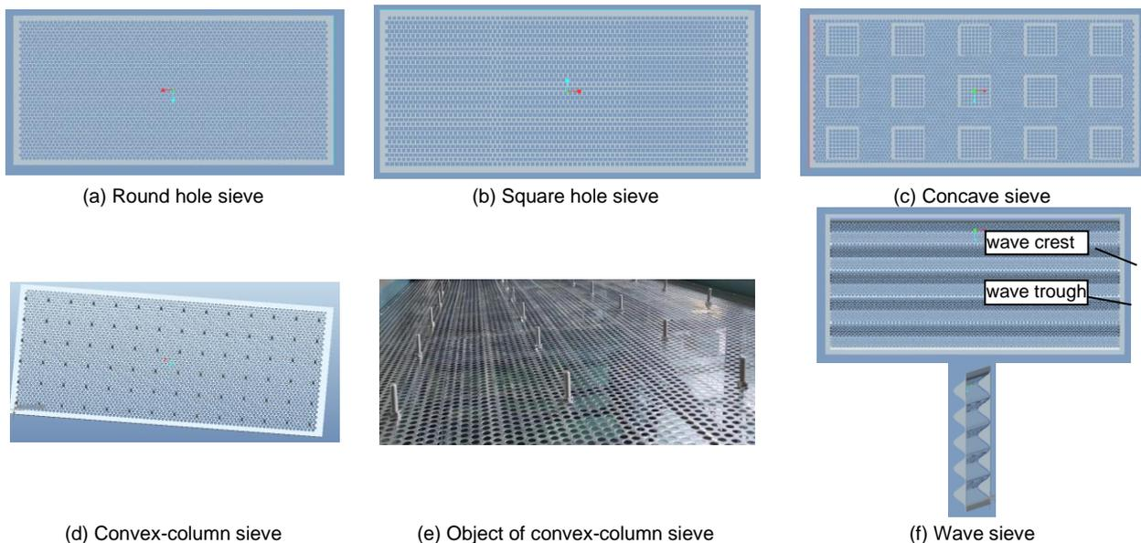
Fig. 3 - Physical models of vibrating screen
