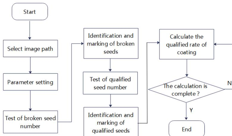
Fig. 11 - The system work flow chart
