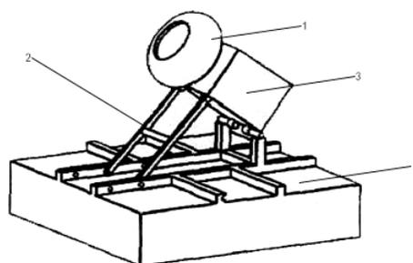
**Fig.1 - The overall structure of seed coating machine**
