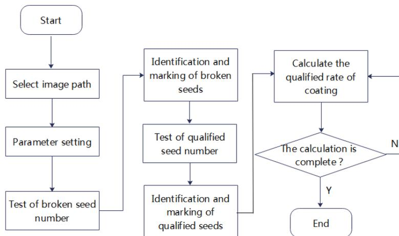
Fig. 11 - The system work flow chart
