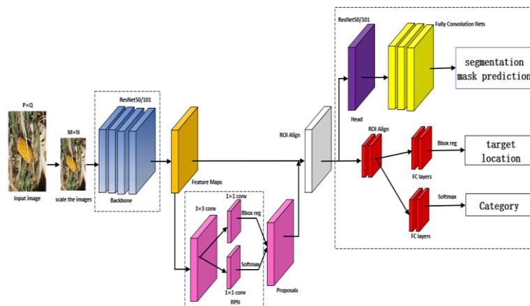
Fig. 3 - Network structure of Mask R-CNN
