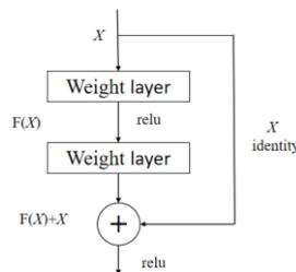
Fig. 6 - Schematic diagram of residual structure
