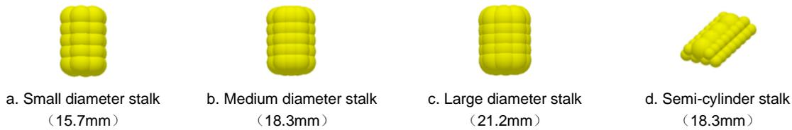
Fig. 2 - DEM model of KG stalk
