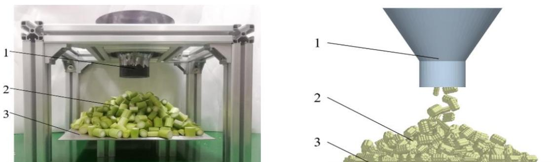
**Fig. 9 - Stacking test of KG stalk**
