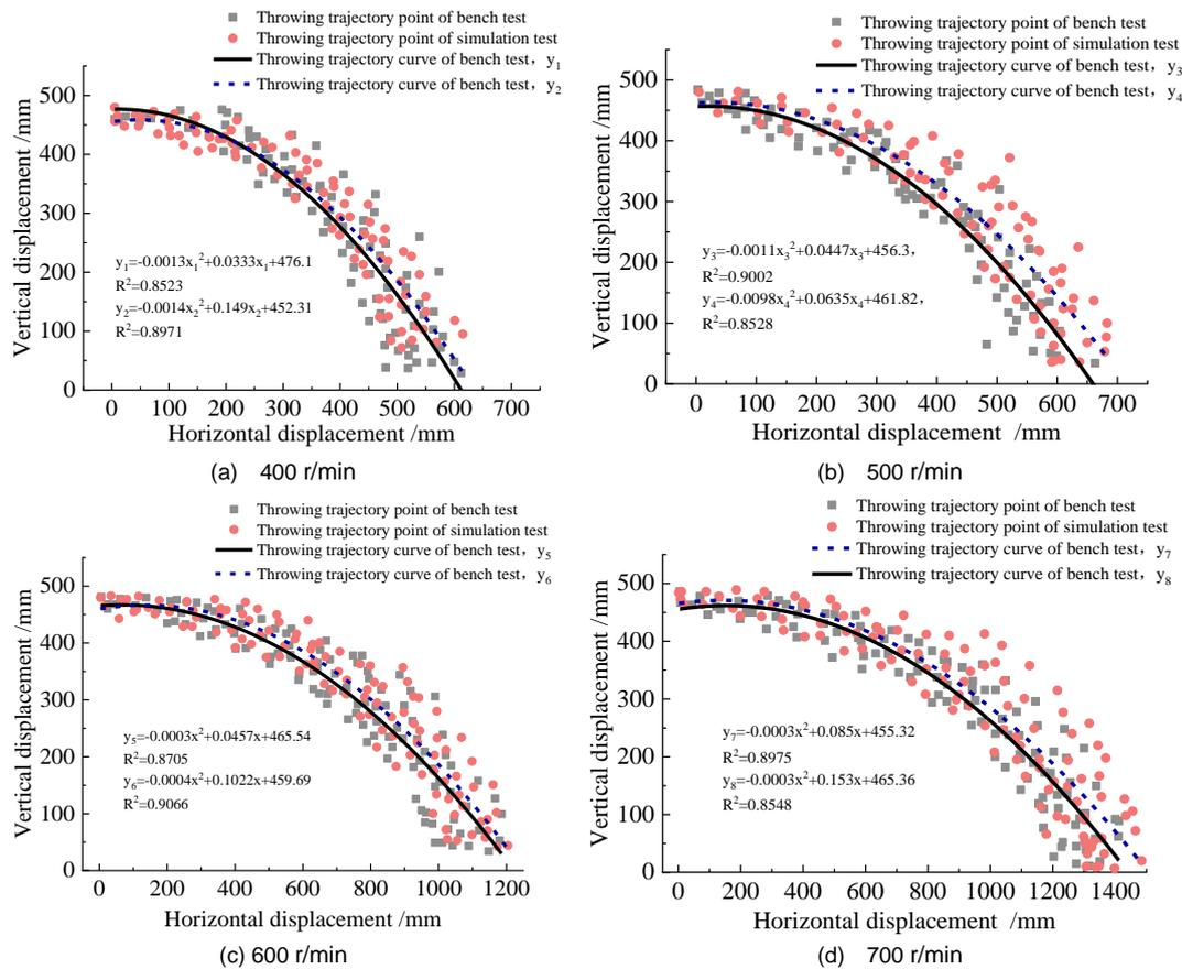
Fig. 14 - Fitting curve of stalk throwing trajectory
