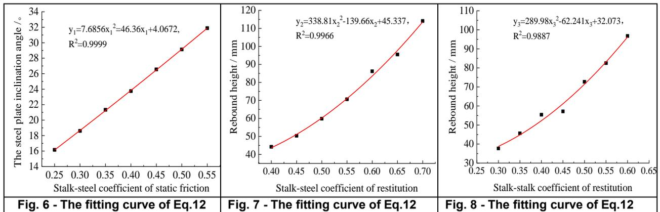
**Calibration of contact parameters based on stacking test**
