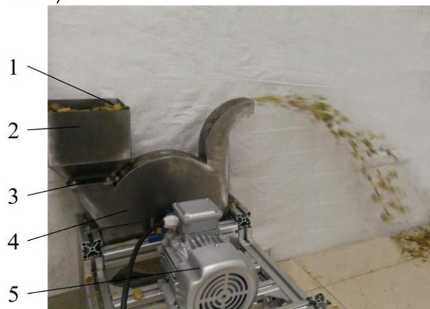
Fig. 11 – Test bed for KG throwing
