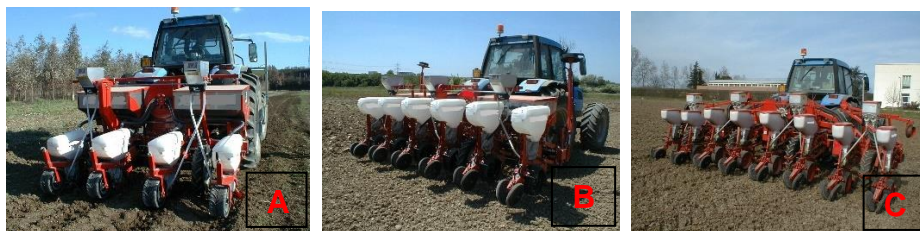
Fig. 1 - The precision drills used in the tests. (A) with four sowing units; (B) with six sowing units; (C) with eight sowing units
