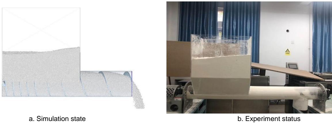
Fig. 14 - Comparison of simulation experiment and real experiment of two dead zone screw feeders (t=10 s)
