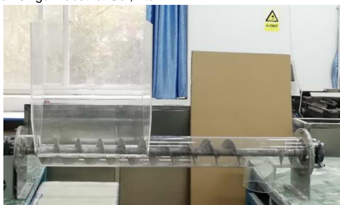
Fig. 7 - Screw feeding experimental platform
