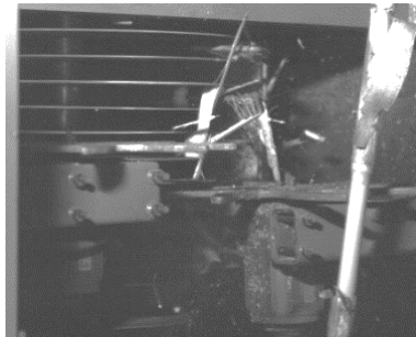
d) The lower part of the stalk was cut by the sawtooth blade group
