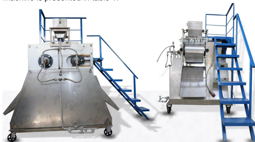
Fig. 6 - The prototype of a double drum dryer
