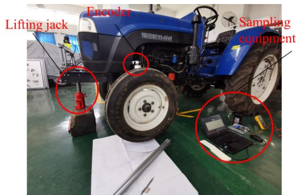
Fig. 6 - Calibration of the tractor front wheel angle via the line drawing method
