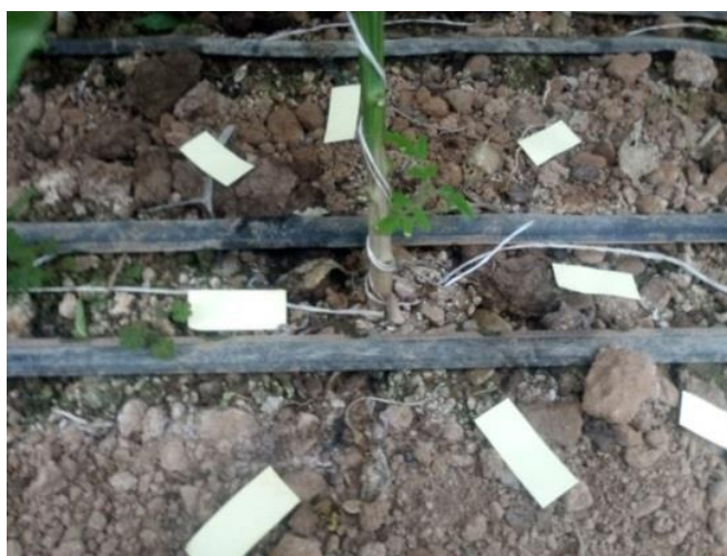
Fig. 8 - Position of sensitive cards to measure spray loss
